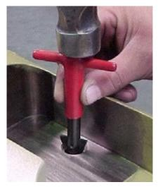
Apply pressure downward with the removal tool located in the two indentations, and turn counter clockwise until the thread is out of the body.
