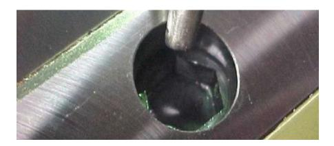
Find the In-hex socket that comes with a new redress kit. Size will depend on the redress kit being used. Place it in the center wedge hole. Push the In-hex socket down until you are sure it is at bottom. With the square drive bar attached turn anti-clockwise until you can remove the wedge from the cartridge.
